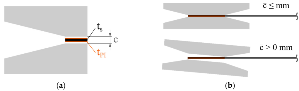
Figure 5. Illustration of the specimen ends positioned in the fixture: (a) theoretical initial situation and (b) effect of the effective gap \bar{c} in the start phase of a test.
