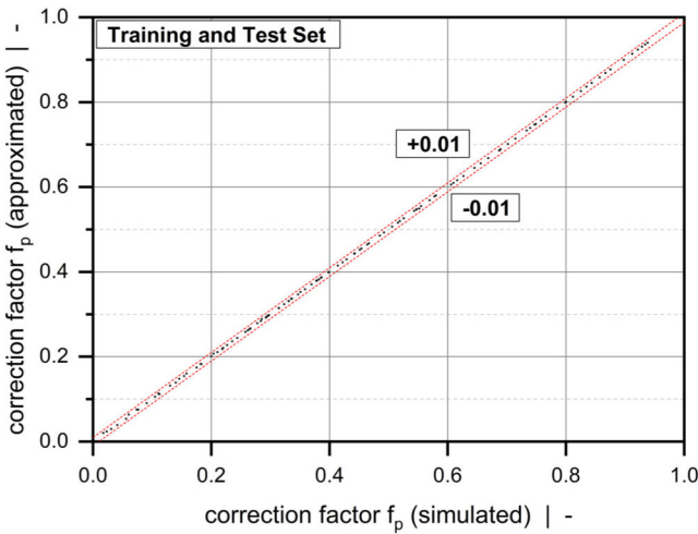
FIGURE 10 Scatter plot of f_p : Comparison between numerical and analytical solutions according to Equation (40). The dashed lines indicate absolute errors.
