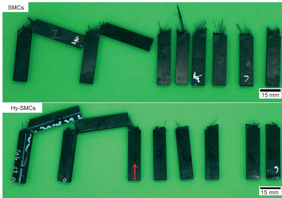
Figure 12. Photographic image of notched Charpy impacted tested SMCs, and the red arrow in Hy-SMCs indicate fibre direction in Hy-SMCs specimens.
